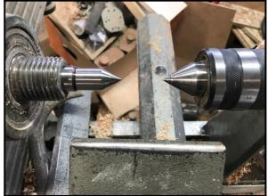
Once you try this method I am sure you will find it most useful as a spindle drive system. For small spindle work I find myself using a 60° center drill to mark the centers of the spindle and turn between these 60° center recesses; it is often an easier method of holding the work than using a stub center or spur drive and has the advantage of being a friction slip drive so that if you have a catch it won't be as serious as it might have been with a spur drive.
